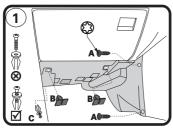
1: Remove 2 screws (A) using special tool, remove 2 clips (B), remove toggle bolt (C) then remove cover.
