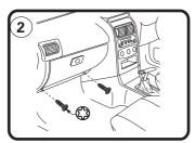
2: Remove 2 screws from bottom of glove box using special tool.
