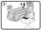
3: Disconnect electrical connection "A" then remove glove box.
